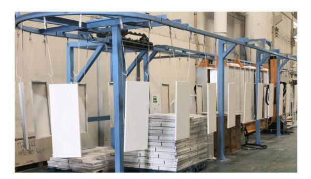
Due to the limited space of plant, we designed an non-continuous line but with automatic powder spraying, including individual pretreatment(dipping), automatic powder coating equipment & automatic powder booth, individual curing oven. As there are some colors to apply, the booth system is designed with cyclone separator, and connects with a powder center for fast cleaning and color change.
